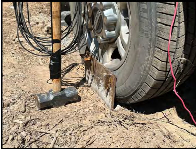
Figure 1. Truck positioned on the source impact plates at DHS23-04
