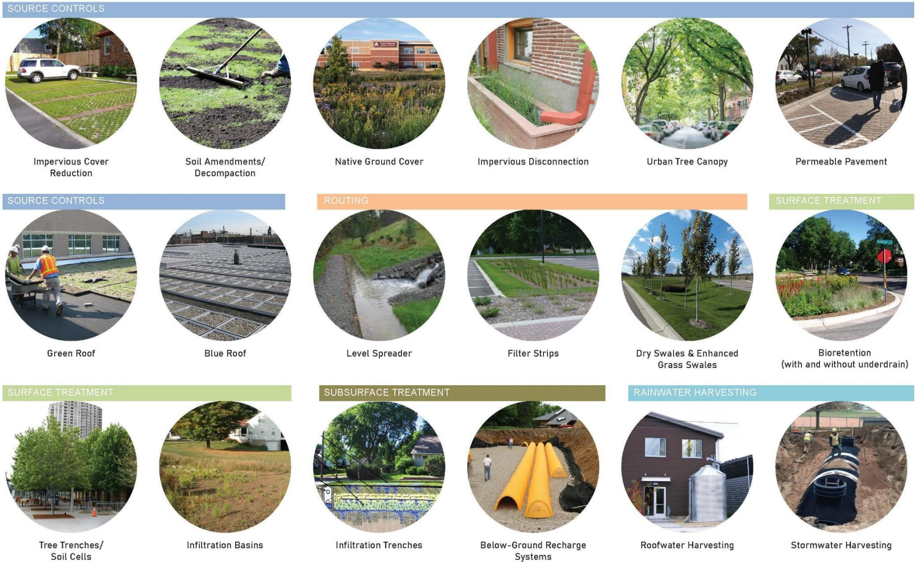
Figure 6: Green Infrastructure Rainwater Management Techniques
