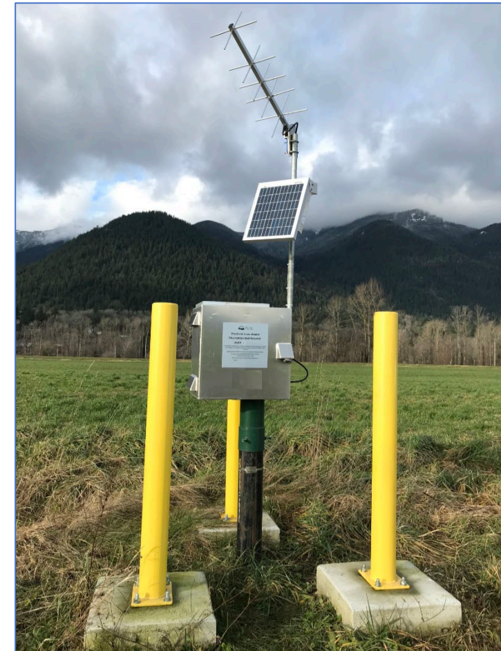
Provincial monitoring well - Monitoring Aquifers: Provincial Groundwater Observation Well Network - Province of British Columbia (gov.bc.ca)
