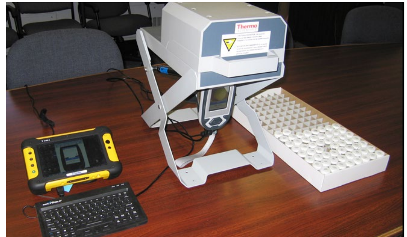
Figure 2.6.1. Portable spectrometer (Thermo Scientific, Niton XL3t GOLDD) used to acquire geochemical data.
