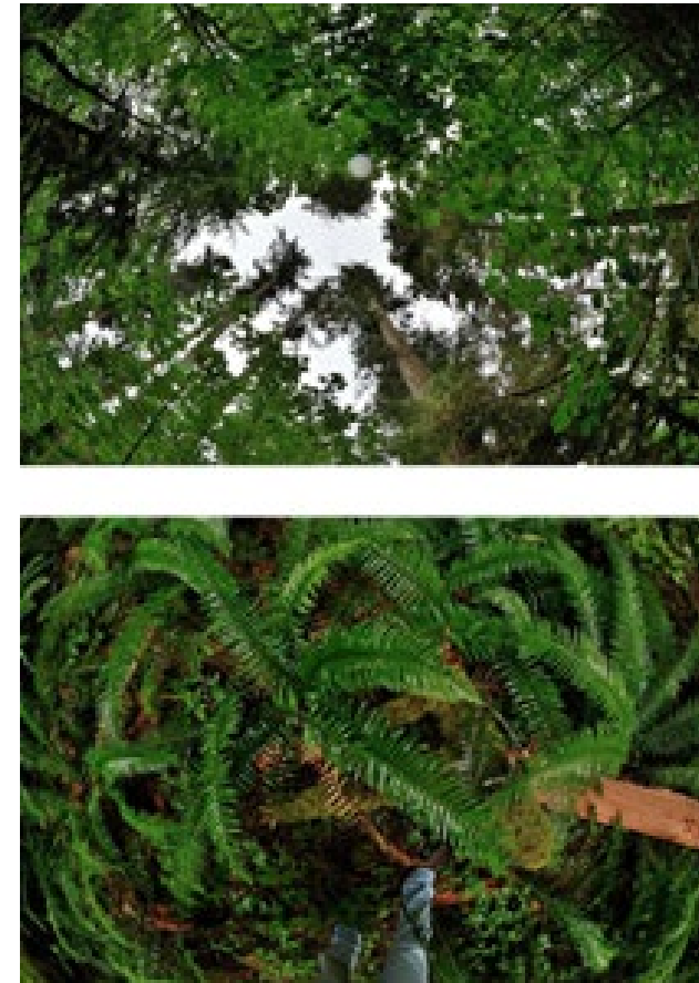
Figure 3.2.1. Up-looking and down-looking hemispherical photograph for overstory and understory leaf area index (LAI) estimation.
