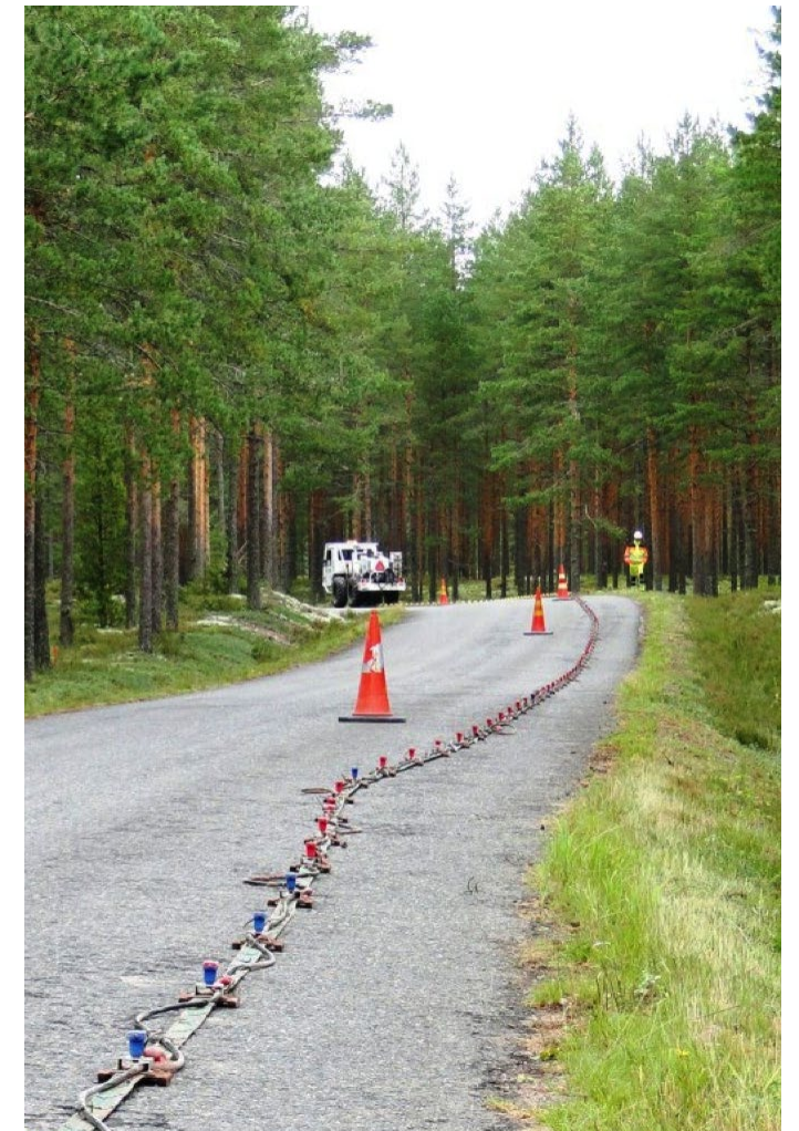
Figure 4.3.2. Vibroseis towing land streamer array of geophones.
