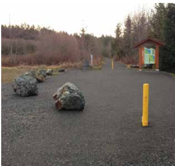
Boulders provide a natural form of bollard
