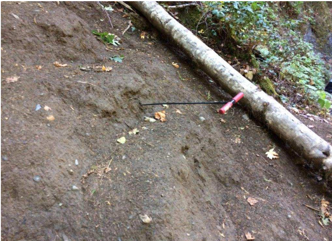
Photo 1: Descent to Ammonite Falls – Probe barely penetrating into soil at heavy foot traffic area.
