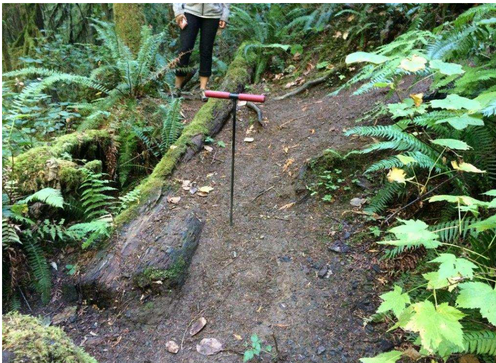
Photo 4: South slope probe in likely foundation area.
