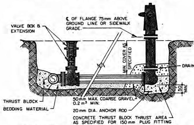
HYDRANT CONNECTION WITH THRUST BLOCK
