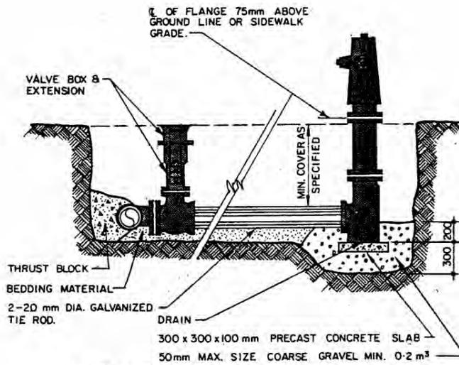
HYDRANT CONNECTION WITH TIE RODS
