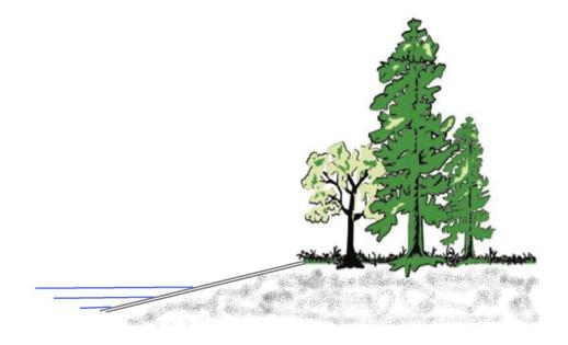
Low angle, stable slope, compact material - low erosion risk
